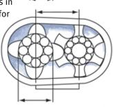
Gas end size determines bearing size
