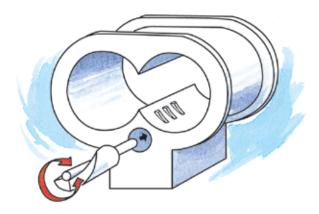
Unneeded gas that has entered the cylinder is allowed to return to the inlet before being compressed.
