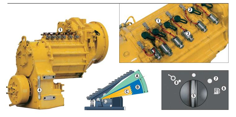
**Electronic power shift transmission with automatic shift capability** is designed, developed and built by Caterpillar. The electronically controlled power shift transmission allows full-power, speed and directional changes. Fully modulated gear shifts significantly contribute to the operator comfort and increase machine productivity as well as component life.
