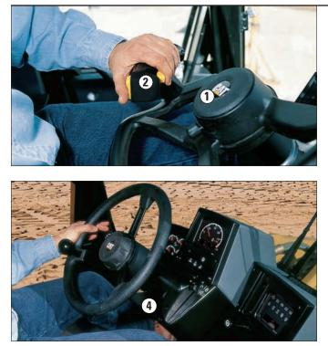
The 950G is available with two different configurations of operator controls – one with Command Control steering and electro-hydraulic implement controls, and another with Conventional steering and pilot hydraulic implement controls.
